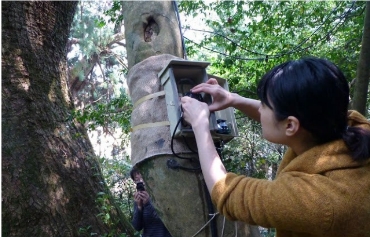
Fixing a sensor measuring bioelectric potential to a tree (Morotsuka, Miyazaki Prefecture)
